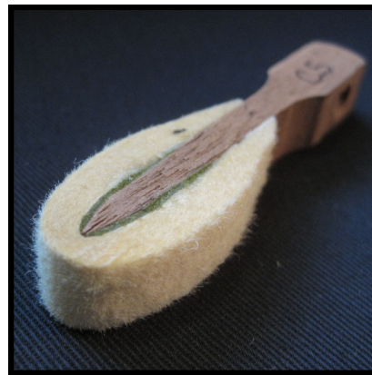
Same hammer after reshaping.
