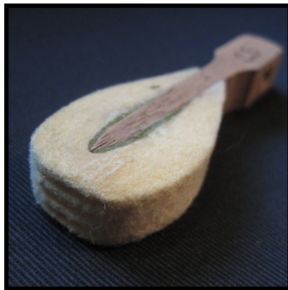
Hammer with significant wear.
